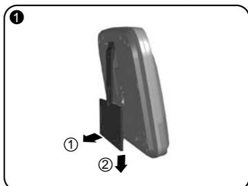
Separate the wall mount from the transmitter.
