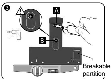
Fix the wall mount with the 2  $\varnothing$  4 mm max. screws by using holes A and B.
