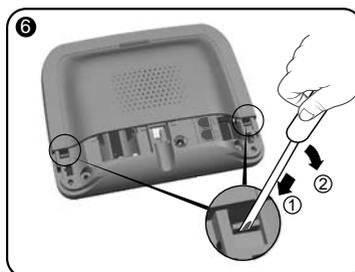
Using a screwdriver, lift the 2 clips of the top cover.
