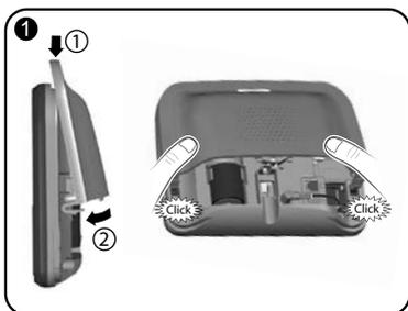
Refit the upper cover and clip it onto the unit.
