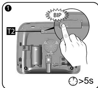
Press the T2 button of the transmitter for 5 seconds.
