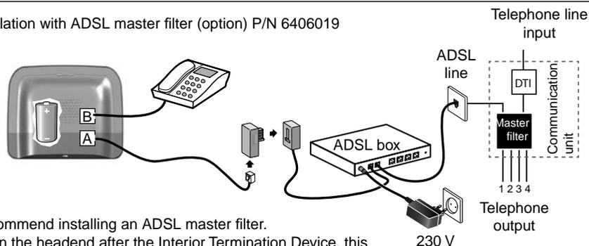
We recommend installing an ADSL master filter. Fitted on the headend after the Interior Termination Device, this device greatly reduces electromagnetic disturbances by separating the ADSL signal of the telephone line. It improves the cohabitation of different devices connected to your telephone installation.
