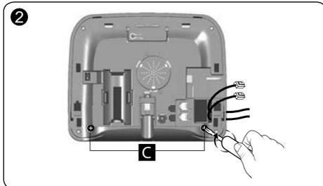
Fix the unit with the 2 Ø 4 mm max. screws by using the C holes.
