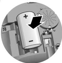
Insert the battery, observing the right polarity.
