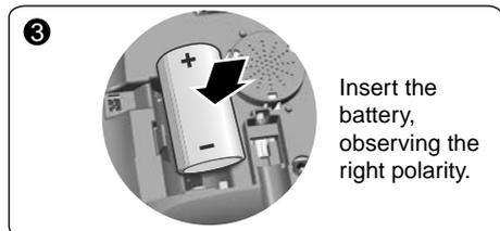
Insert the battery, observing the right polarity.
