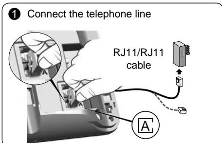
Connect the RJ11/RJ11 cable to the telephone line inserting the RJ11 adapter suitable for your installation.
